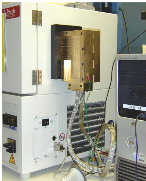
FIGURE 1. A modified thermal chamber contains a shielded adapter for RF cables and digital control cables.
